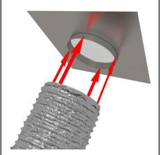
Slip the flexi shaft over the metal collar on the underside of the skylight dome.
